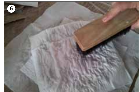
6 Using the brush, tap thoroughly on the last layer.
