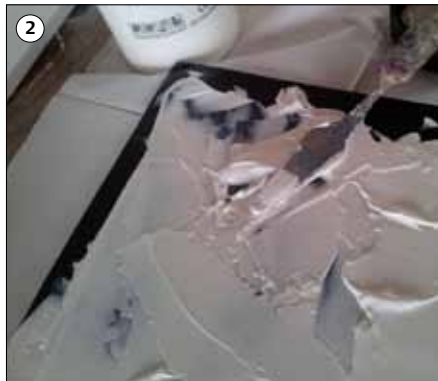
2 Spread a thick layer of ReliefBase onto the item.
